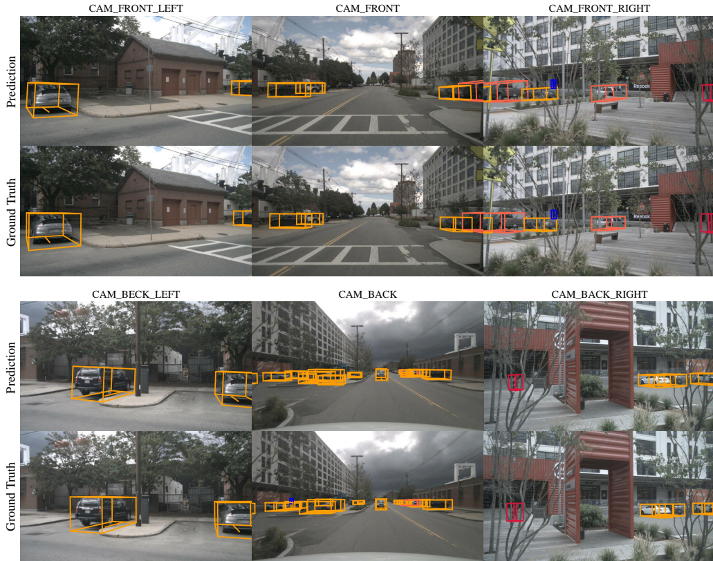
Figure 4. Visualization of BEVFormer v2 3D object detection predictions.
