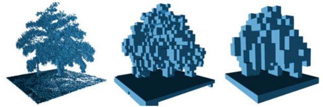
Fig. 3 By limiting the depth of a query, multiple resolutions of the same map can be obtained at any time. Occupied voxels are displayed in resolutions 0.08, 0.64, and 1.28 m
