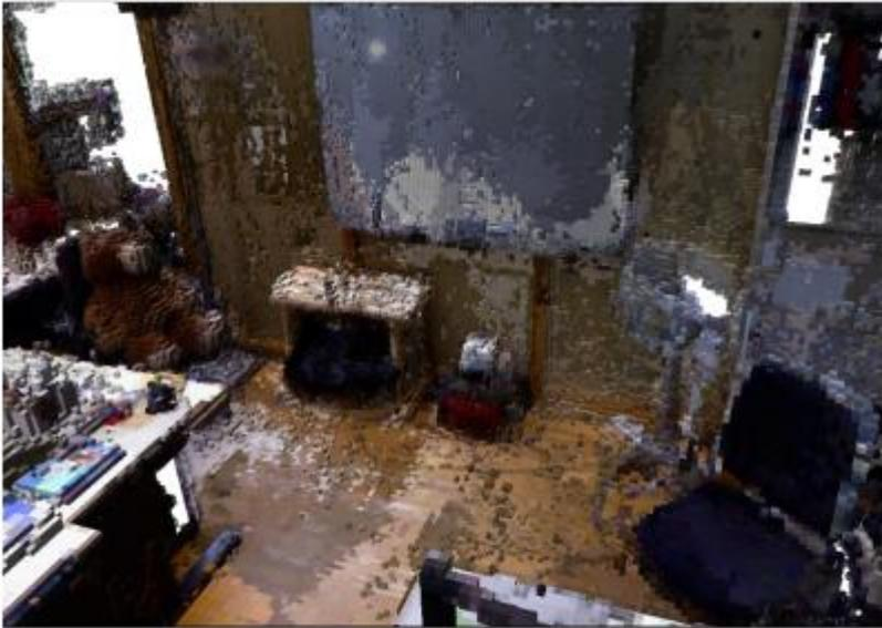
**Fig. 5** Detail of a volumetric indoor OctoMap containing color information. The complete map covers an area of  $7.3\text{ m} \times 7.9\text{ m} \times 4.6\text{ m}$  at  $2\text{ cm}$  resolution. [https://blog.csdn.net/weixin\\_36652031](https://blog.csdn.net/weixin_36652031)
